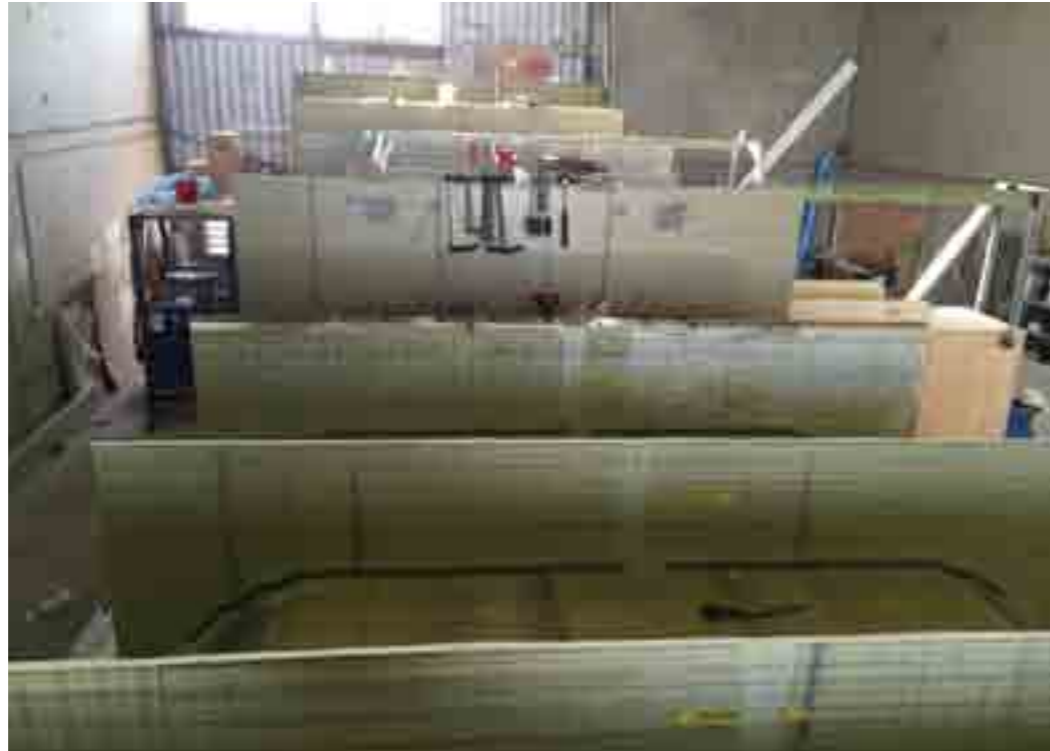
After extensive testing a new system is being used to bond in the bulkheads and other structures.
