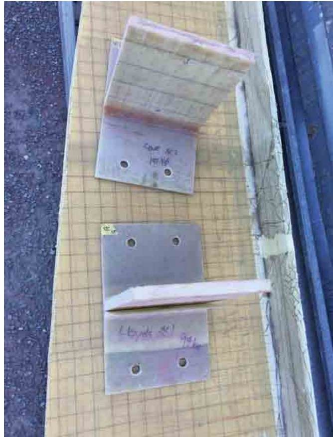
Tests comparing a standard Lloyds tabbed bulkhead join with a Crestomer 1152PA coved join demonstrate that the coved joint is over twice as strong
